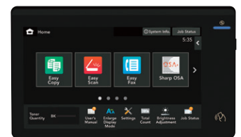
10.1" (diagonally measured) customizable touchscreen display.
